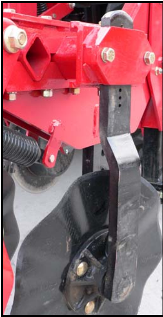
Rigid Mount Three Adjustments
