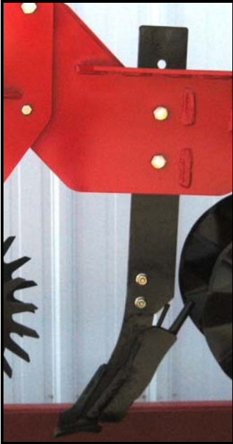
Shear Bolt Protected Shank
