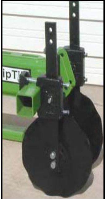
Two Way Blade Adjustment
