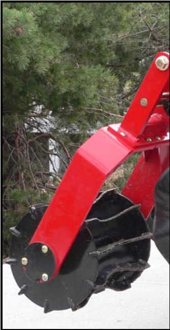
Concave Reel and Faster Reel Speed
