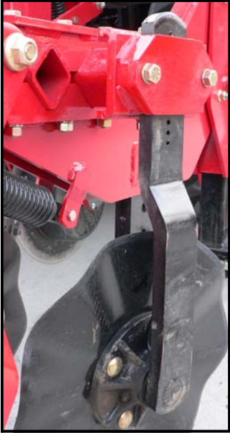
Positive Positioned Wavy Blades
