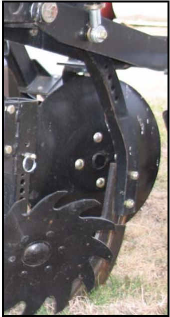
Curved Chisel Plow Style Shank
