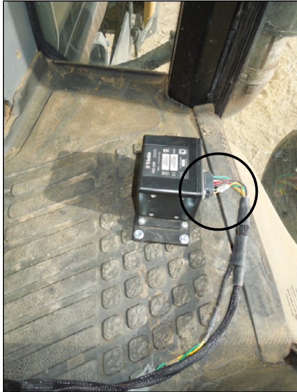
Example installation: IMD-600 cable connection Ford / New Holland / Buhler / Versatile front wheel steer tractors and CAT tracked tractors
