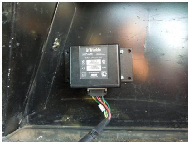
Example installation: IMD-600 cable connection Ford/New Holland/Buhler/Versatile articulated tractors
