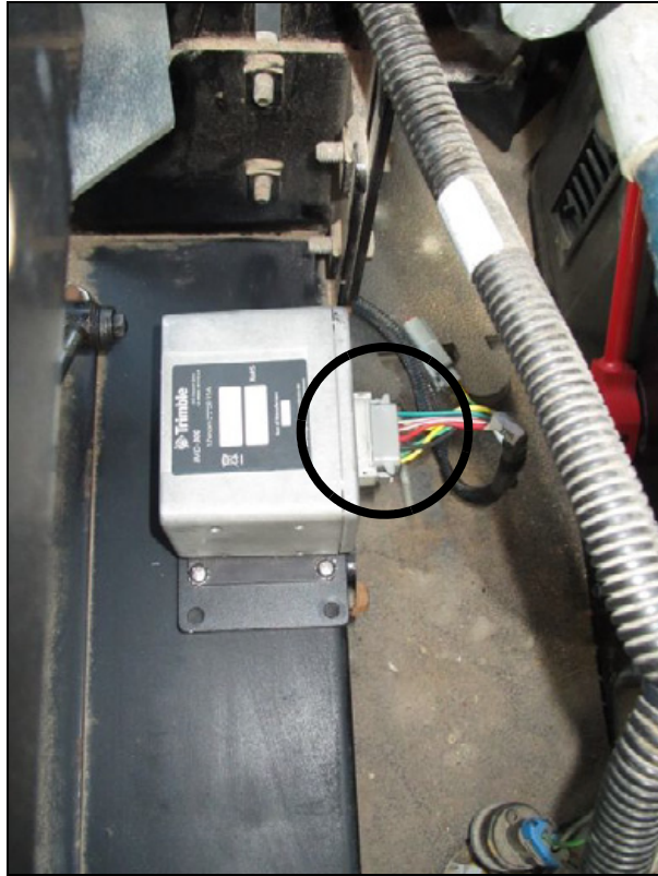
Example installation: IMD-600 cable connection AgChem TerraGator floaters / Rogator sprayers
