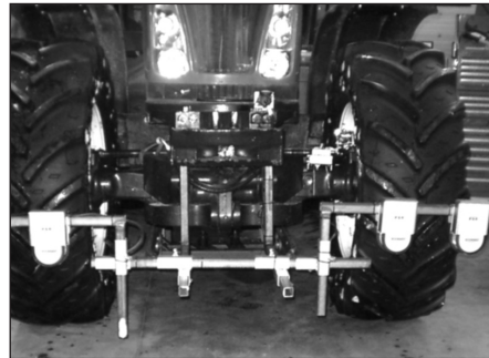
Picture 11: Sonic sensors side by side
