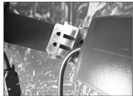
Picture 9: Slide RDU into the mounting slider
